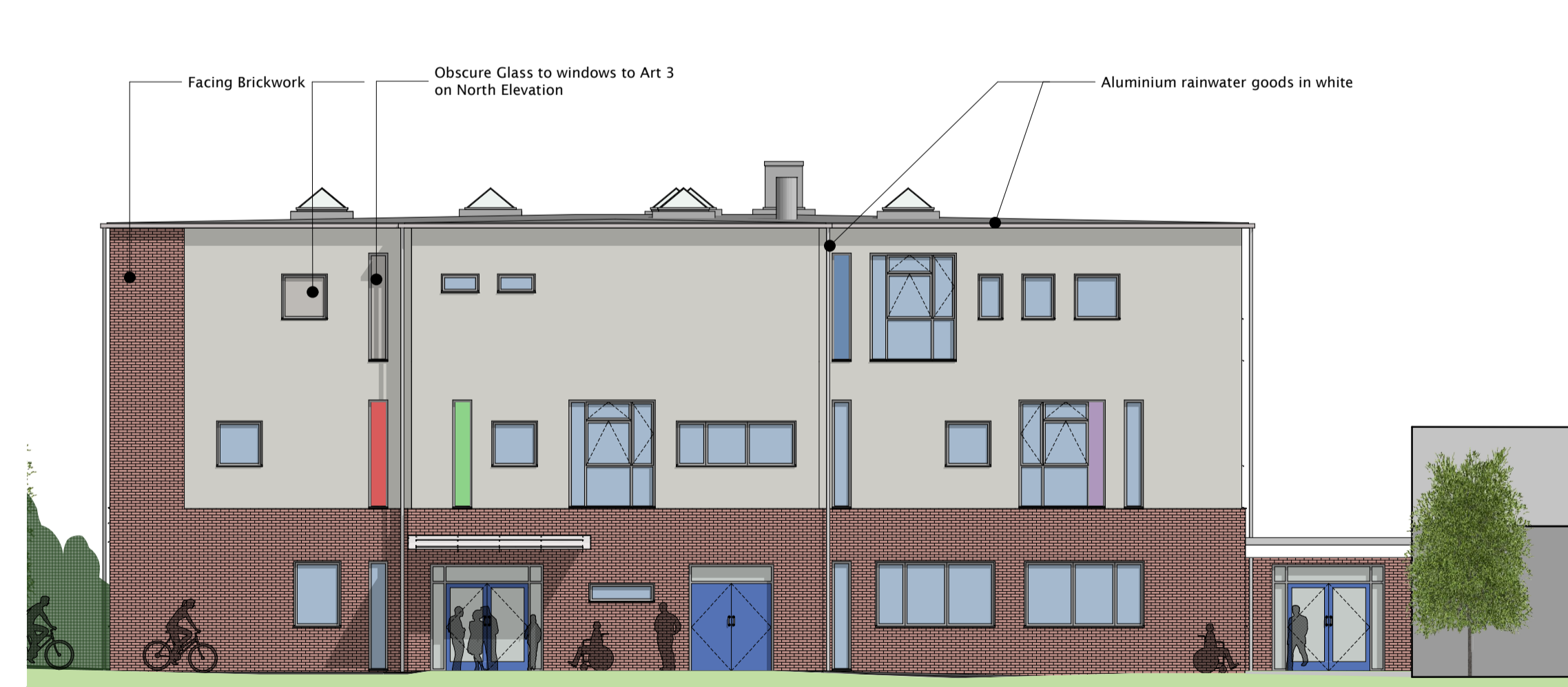
New Extension North Elevation
